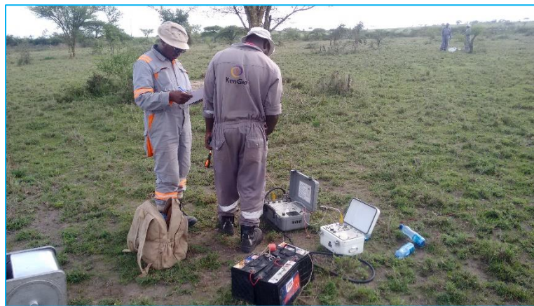
Figure 27. Set up of TDEM system (KenGen), transmitter with car batteries at the corner of the Transmitter loop (100x100), the receiver and the multi coil receiver antenna are in the center (at distance).
