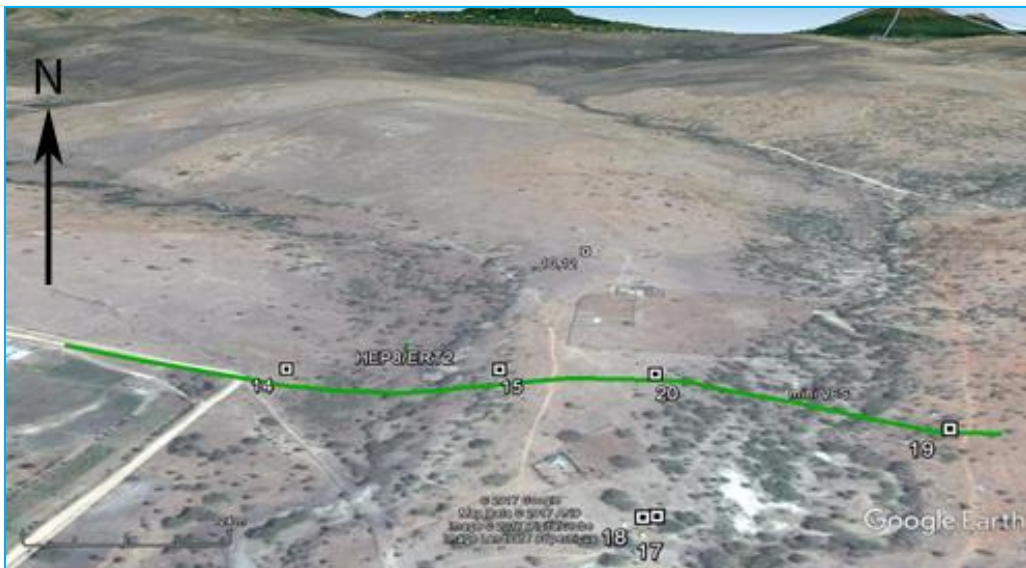
Figure 51. Location of the ERT /HEP profile (green line) and the VES sounding locations (boxes) at Kajiado River profile
