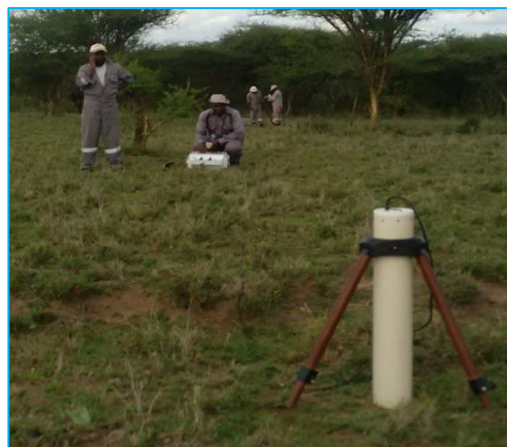
Figure 28. Detail of the carefully oriented TDEM multi coil receiver antenna. In the back the (Zonge GDP32-II) receiving instrument, and further away (near the trees), the location of the (Zonge ZT30) transmitter at the corner of the insulated single copper wire transmitter antenna loop which is laid down in a square around the set up. The receiver antenna is located in the center of the transmitter loop.
