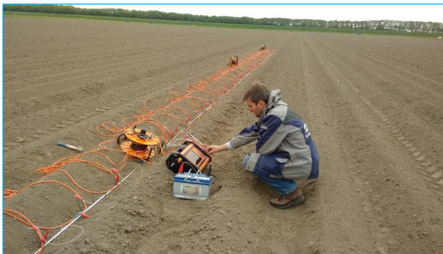
Figure 17. Overview of ABEM ERT instrumentation: four reels are interconnected, with in the center an ABEM Terrameter LS. This photo was selected because of the good overview. The location was in the Netherlands, electrode distances were very short in order to monitor the development of shallow fresh water lenses over time due to new irrigations systems. Exploration depth with this set up is only 7 meter, with a very high resolution.
