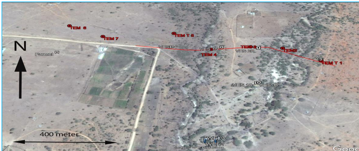
Figure 49 Location of Kajiado river profile on a North-up Google Earth overview, the red line is the ERT profile; this was also the HEP profile. Red dots indicate locations of the TDEM (and AMT) stations used in inversions. The white boxes are the VES locations
