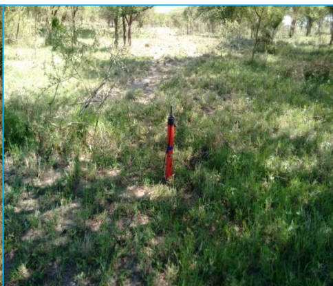
Figure 42. Vertical oriented Magnetic coil
