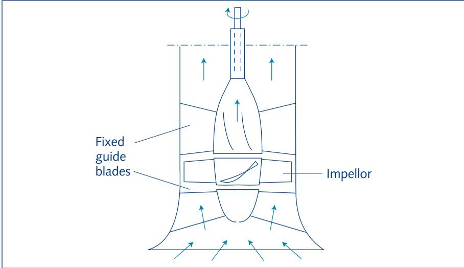
Fig. 9.14. Axial-flow pump
