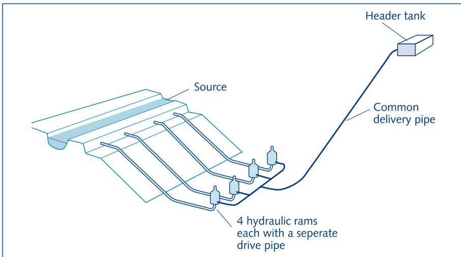
Fig. 9.22. Hydraulic rams placed parallel.
