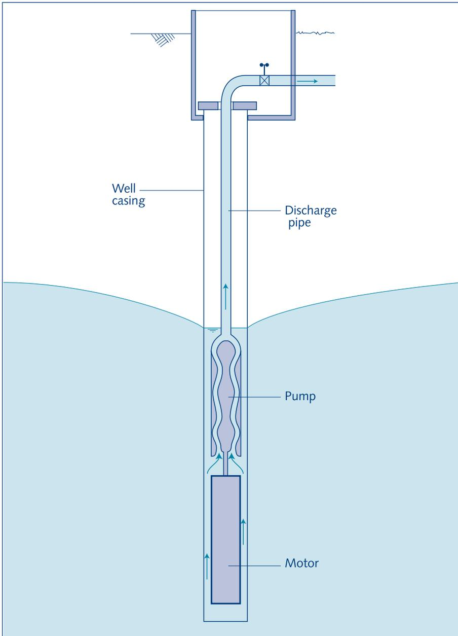
Fig. 9.17. Pump driven by a close-coupled submersible electric motor
