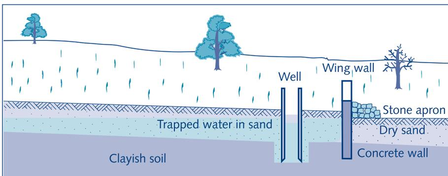
Fig. 6.20 Sub-surface masonry dam (Adapted from Nissen-Petersen, E., 1986)
