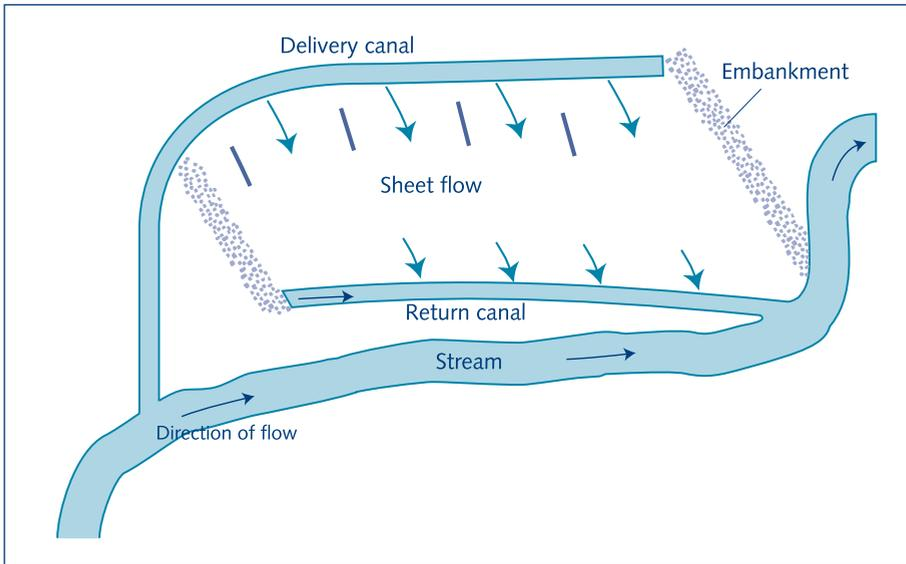
Fig. 6.2. Flooding technique
