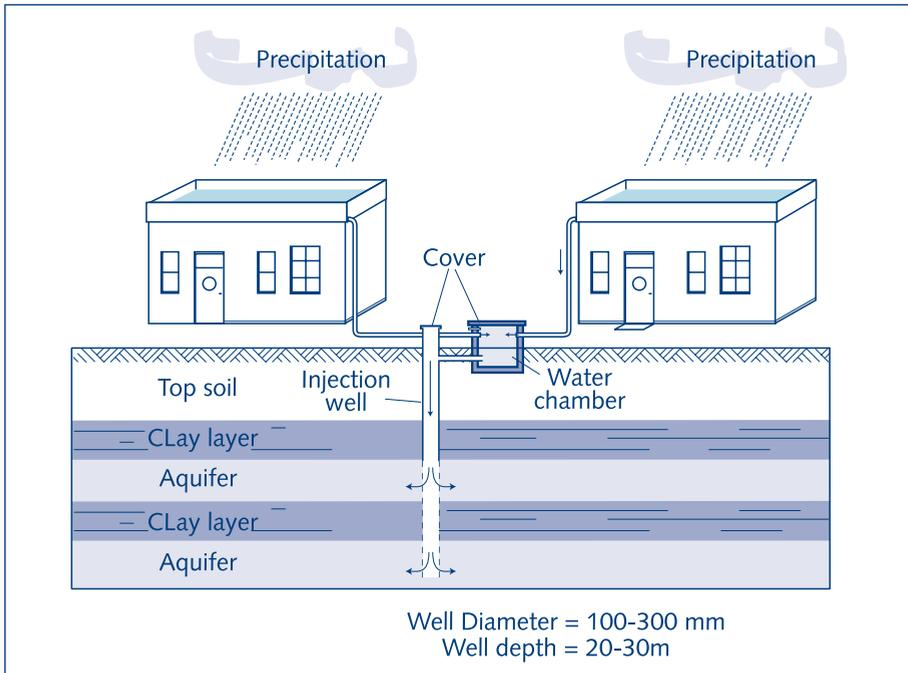
Fig. 6.16. Gravity head recharge well or borehole
