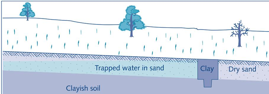
Fig. 6.19. Sub-surface clay dam (Adapted from Nissen-Petersen, E., 1986)
