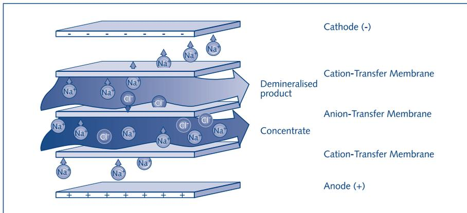
Fig. 18.7. The electrodialysis process
