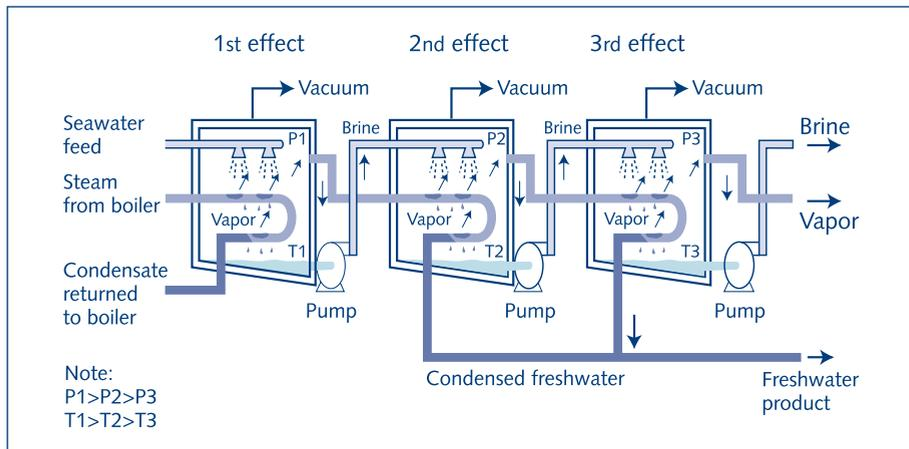
Fig. 18.1. Schematic diagram of a multi-effect distillation (MED) unit
