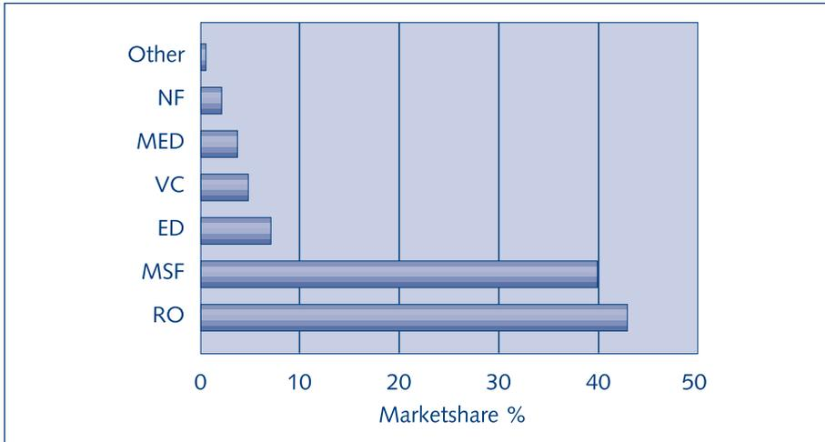
Fig. 18.8. Market share of thermal and membrane processes for desalination plants in operation
