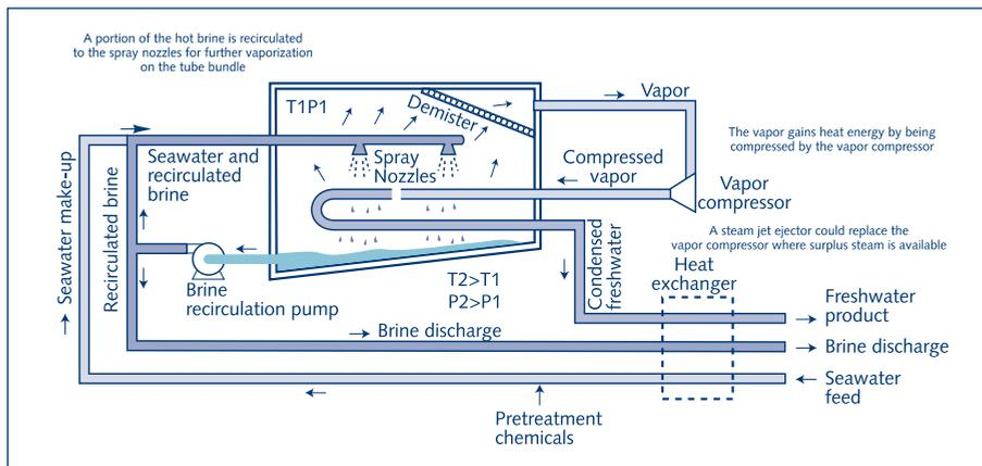
Fig. 18.5. Schematic diagram of a vapour compression (VC) unit
