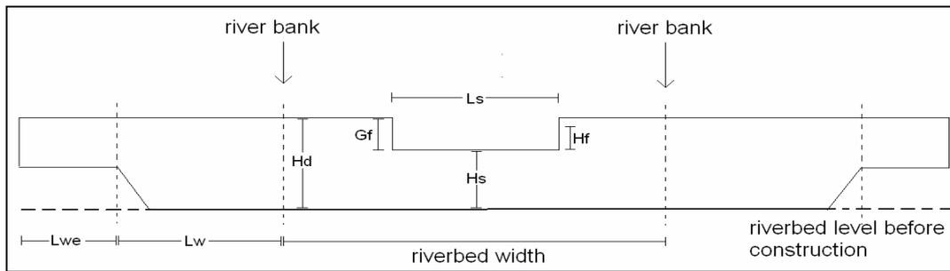
**Figure 10:** Cross section of a sand dam body and its dimensions.
