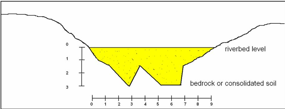
**Figure 7:** Example of cross profile and probing results.
