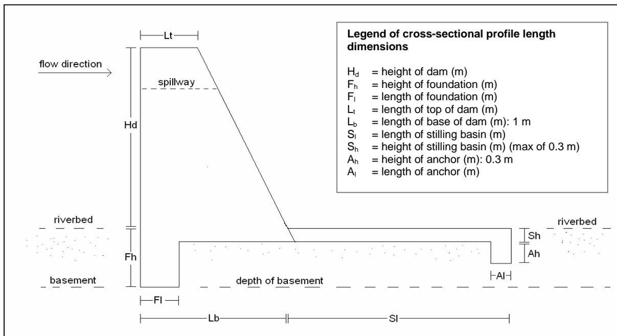
**Figure 11:** Cross sectional profile of a sand dam body and its dimensions.
