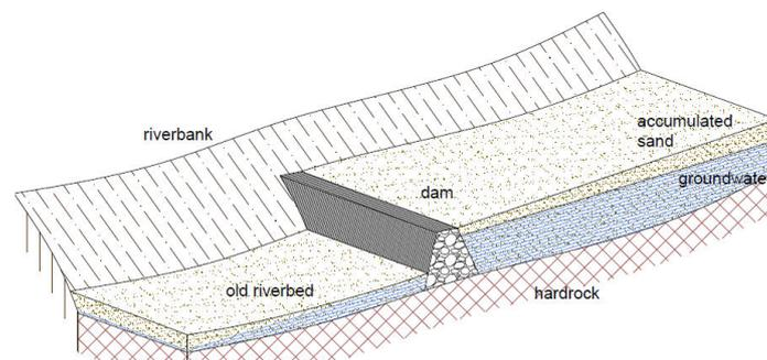
**Figure 2:** Schematic cross section of a typical sand storage dam (Borst & de Haas, 2006)
