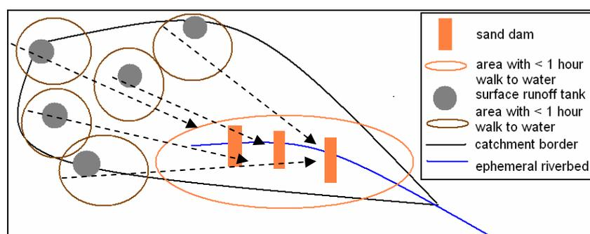
**Figure 1:** Hypothetical example of catchment approach in rainwater harvesting: combining sand dams and rainwater harvesting tanks in one (sub)catchment.
