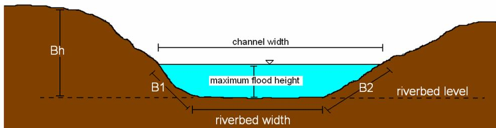
**Figure 9:** Cross section with maximum flood height to determine maximum discharge.
