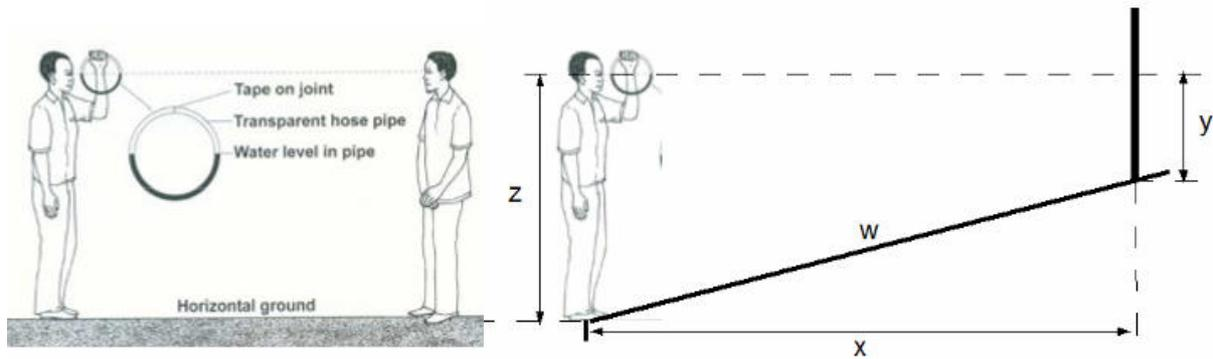
**Figure 5:** Usage of the levelling tool at horizontal grounds (left) and at sloping grounds (right) (Nissen-Petersen, 2006a).
