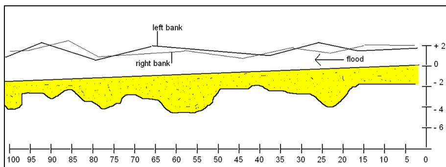
**Figure 6:** Example of a longitudinal profile of a river section.
