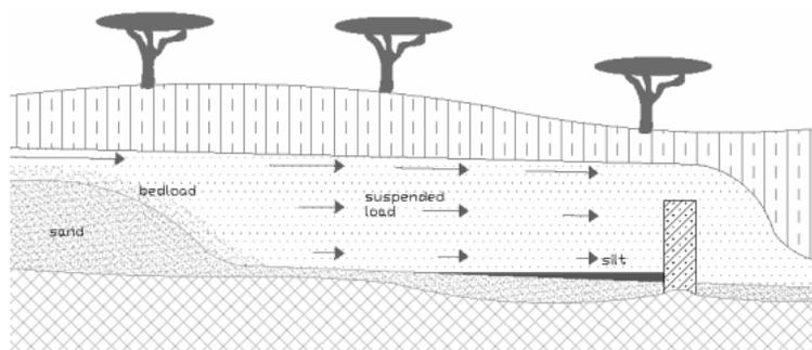
**Figure 3:** Schematic representation of the sedimentation process (Gijsbertsen, 2007)
