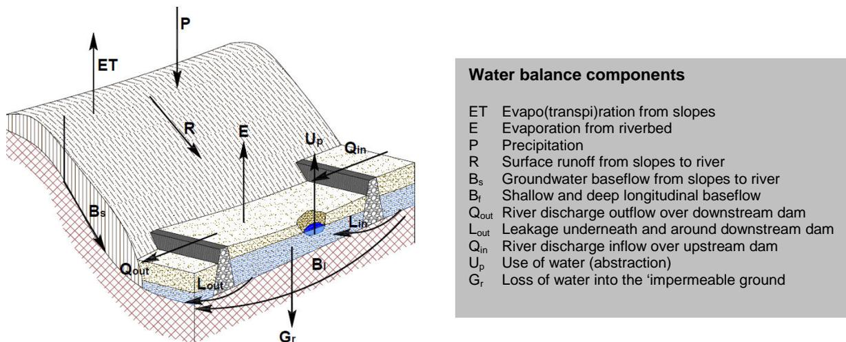
Figure 4: Important water balance components to the hydrological functioning (Borst & de Haas, 2006).
