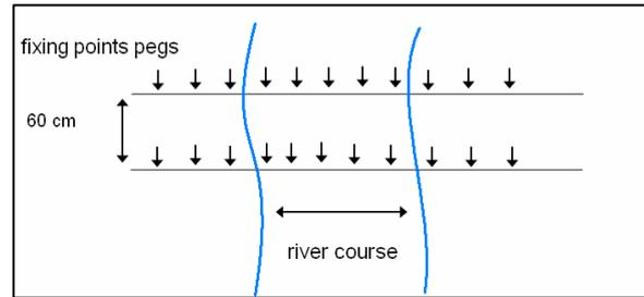
**Figure 13:** Example of setting a trench with pegs.
