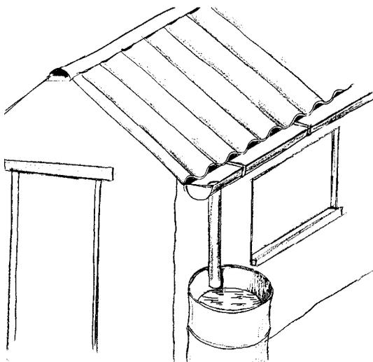
*Figure 1: Rainwater harvesting system*
