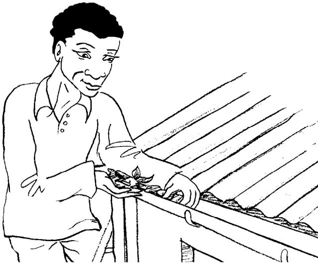
*Figure 30: Remove debris from the gutter system regularly*
