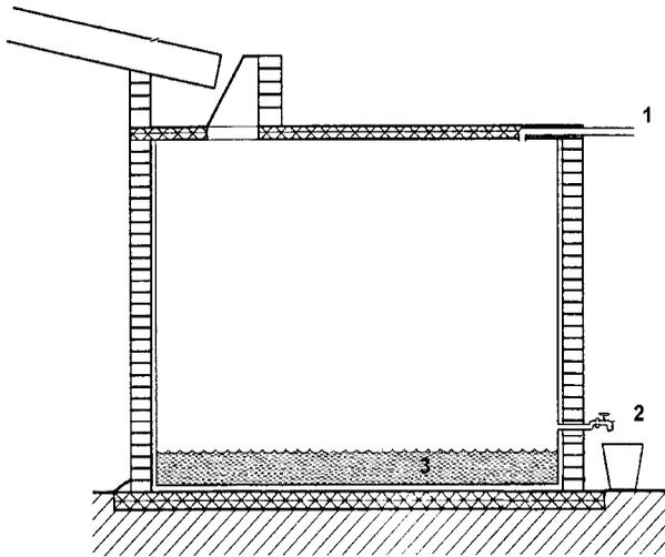
Figure 17: Overflow (1), Tap device (2), Dead storage (3)
