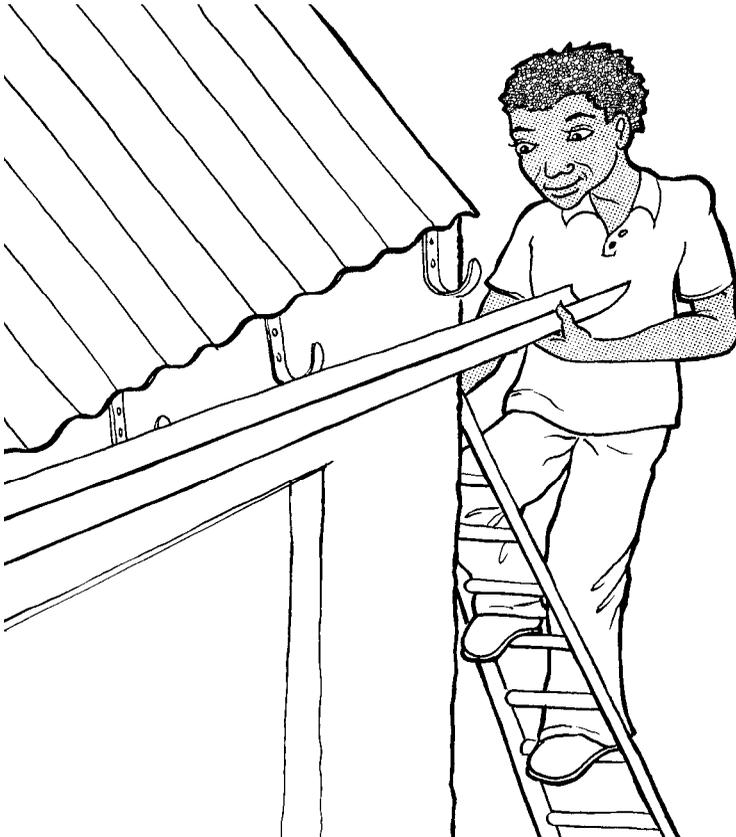
*Figure 4: Connecting a gutter system*
