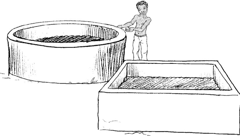
*Figure 6: Storage reservoirs for large quantities of water (from 1 m<sup>3</sup> to 30 m<sup>3</sup> for a domestic system at household level)*
