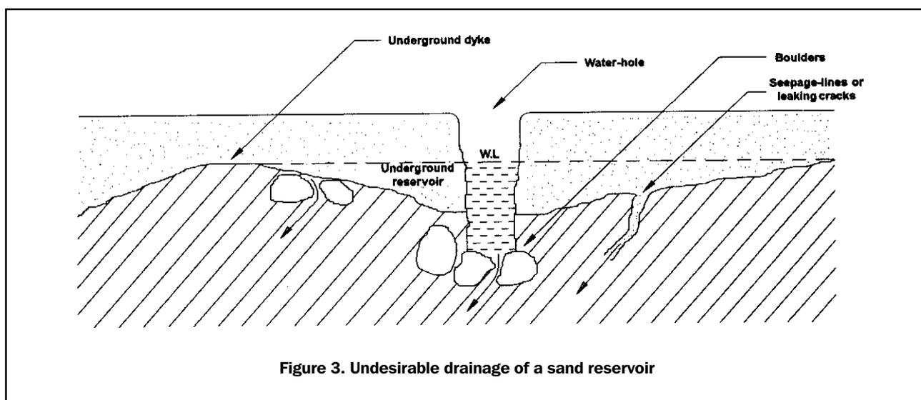
Figure 3. Undesirable drainage of a sand reservoir
