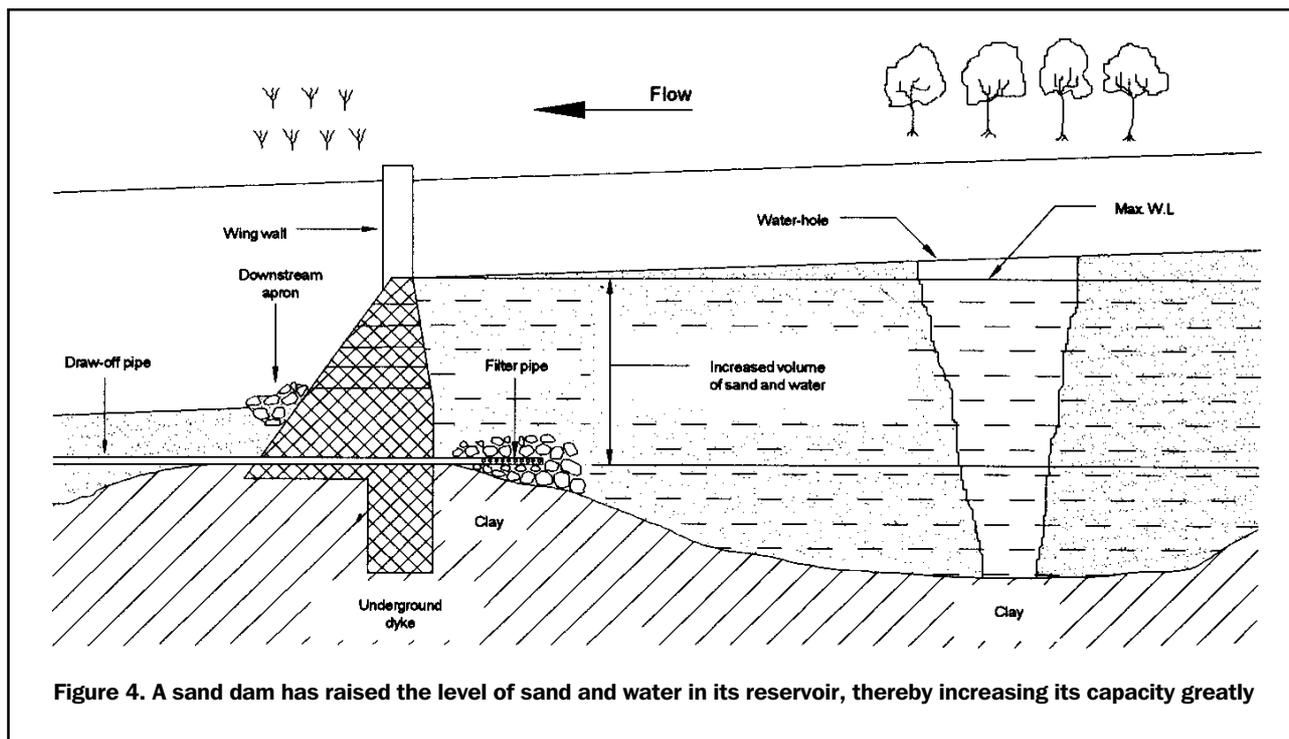
Figure 4. A sand dam has raised the level of sand and water in its reservoir, thereby increasing its capacity greatly
