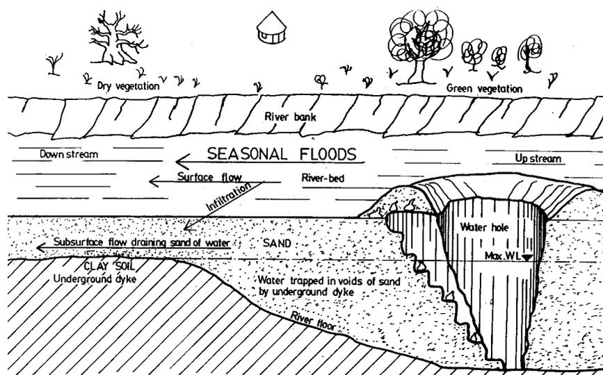
**Figure 1. Longitudinal profile of a sand-river trapping water**
