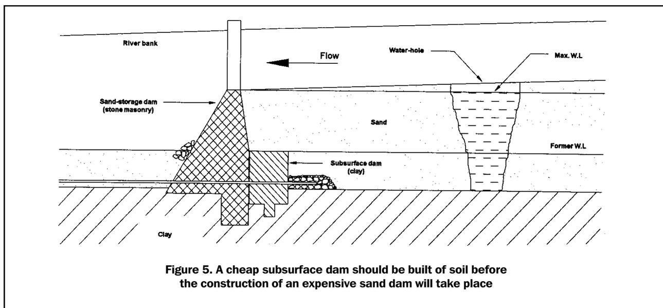
Figure 5. A cheap subsurface dam should be built of soil before the construction of an expensive sand dam will take place
