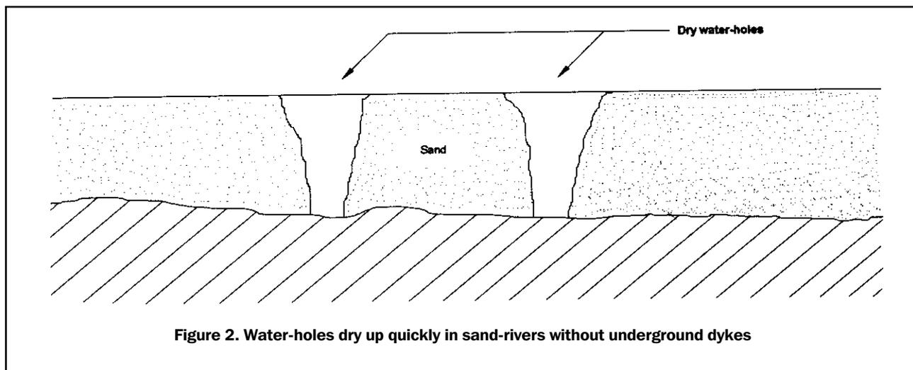
Figure 2. Water-holes dry up quickly in sand-rivers without underground dykes
