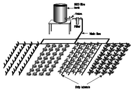
Figure 4.8 Layout of Plastro system.
