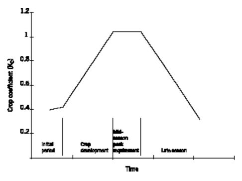
**Figure 2.1** Example of a crop coefficient  $(K_c)$  curve.
