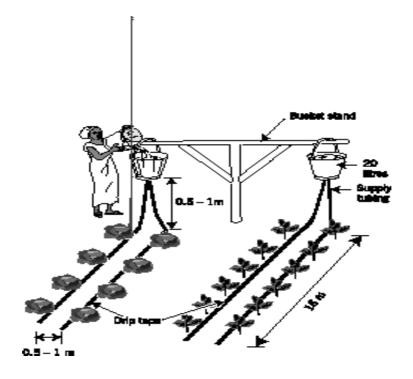
Figure 4.1 Layout of Chapin bucket system with two drip lines.
