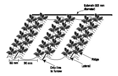
**Figure 4.15** A paired row drip system for cost reduction.
