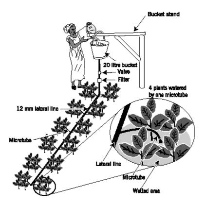
Figure 4.3 Layout of IDE bucket system.
