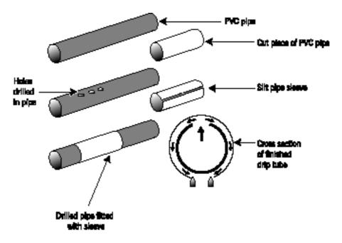
Figure 3.3 Simple drip emitter: a hole and collar.
