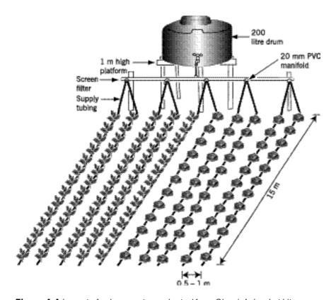
Figure 4.4 Layout of a drum system adapted from Chapin's bucket kit.
