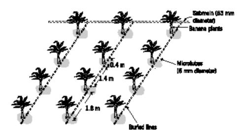
Figure 4.13 Subsurface drip system for banana.
