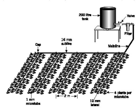
Figure 4.9 Layout of IDE drum system.
