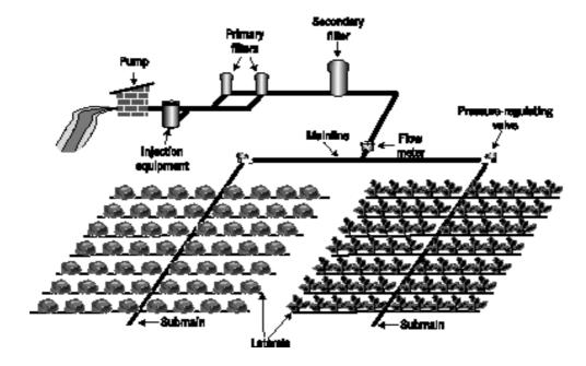
Figure 3.1 A typical drip irrigation system.
