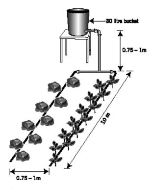
Figure 4.2 Layout of Waterboys bucket system.
