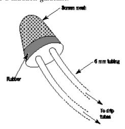
Figure 3.2 Simple filter screen.
